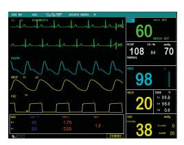
With the multi-gas analysis module, perform 5-agent measurement, along with  $ETCO_2$ ,  $N_2O$  and  $O_2$ , easily and reliably.
